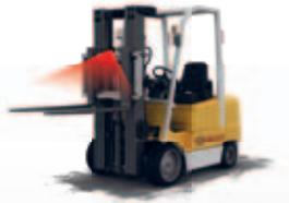
Loading and unloading of trucks often requires the forks to be at a height where the view of the forks is blocked by the fork carriage. The **View-on-forks** system allows the driver to maintain a view of the forks.
