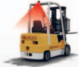
In confined areas or unclear situations it is often difficult to estimate the space behind the forklift truck accurately. Also, frequent driving in reverse causes strain on the driver's neck- and shoulder muscles. The **Rearview** system ensures a safe environment in which the physical strain for the driver is minimal.
